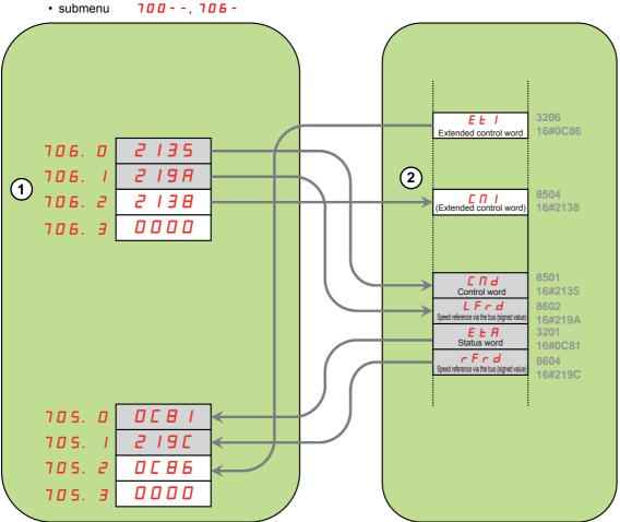
The required telegram to perform the exchange is the Modbus function 23, Obviously a sequence of requests based on Modbus functions 03 and 16 is also possible.
